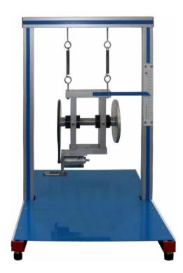
**Simple Balancing Apparatus Model KSM-057** is a unit designed to study and analyze oscillations and vibrations, and to explore methods for eliminating or reducing them.
